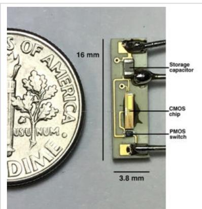
The internal components of a battery-less pacemaker introduced this week by Rice University and the Texas Heart Institute. The pacemaker can be inserted into the heart and powered by a battery pack outside the body, eliminating the need for wire leads and surgeries to occasionally replace the battery. *[Image from Rice Integrated Systems and Circuits/Rice University]*
